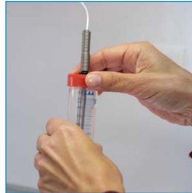
4. Mount the vial in the fridge or freezer accordingly. The vial can be mounted with Velcro, tie-wraps, double-sided tap or the supplied tube holder.
