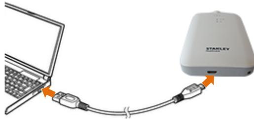
2. Device drivers are automatically installed the first time the device is connected to a PC.
