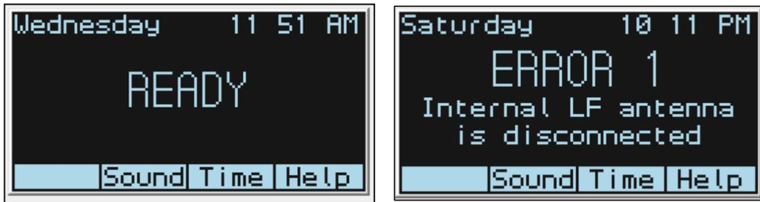
Time and Day of the Week are displayed on the upper row of the LED display. The display shows the mode/status of the Controller and indicates any Controller error such as a communication failure with the Controller.
