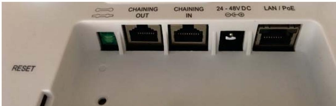
**LAN / PoE:** RJ-45 connector. In a configuration with a physical Ethernet cable connection to the LAN, the network cable is attached here.
