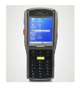
SAAT-H810 is a potable active reader which operates in the 916 MHz band, with high performance, powerful extensible function, flexibility and integration. SAAT-H810 combines the portability and user-friendly together, which is easy to use and complies body engineering. SAAT-H810 is suitable for pet location, asset tracking, traffic vehicle management, etc.
