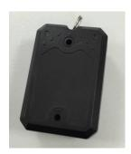
SAAT-T815A Active LED & Beep tag works in 916MHz frequency band in active working mode. The tag has both LED and buzzer to indicate the working status of tags. With waterproof and battery changeable design, the tag SAAT-T815A is very suitable for many application occasions such as pet tracking/asset management/monitoring/locating etc. Waterproofing IP65.
