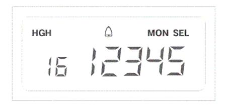
SEL indication at right top of LCD means 5 tone calling mode. Two digits number displayed in small font at left is memory number. 5 digits number in large font represents party's ID number included in the memory. Accordingly, the above example shows a calling number,'12345' and stored number,'16'. You can set and modify these numbers by PC programmer or front panel key.
