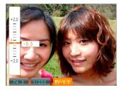
Press Up/Down button to adjust the exposure value of image, with scope from EV -2.0 to EV+2.0.
