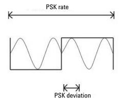
Figure 2-23 PSK modulation waveform
