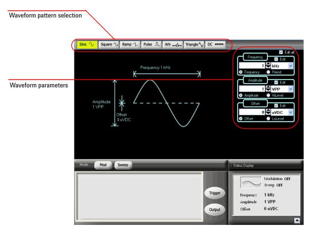
Figure 2-1 U2761A soft front panel
