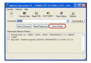
**5** If the Connection Expert can successfully communicate with the U2761A, this indicates that the instrument is installed correctly.
