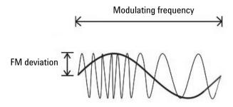
Figure 2-17 FM waveform
