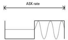
Figure 2-25 ASK modulation waveform
