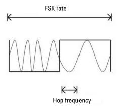
Figure 2-21 FSK modulation waveform
