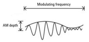
Figure 2-14 AM waveform
