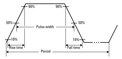
Figure 2-12 Pulse waveform
