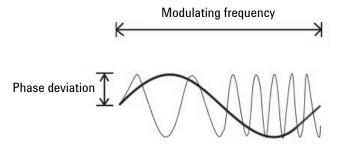
Figure 2-19 PM waveform
