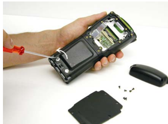
6. Remove the cover from the battery room by unlocking the screws.
