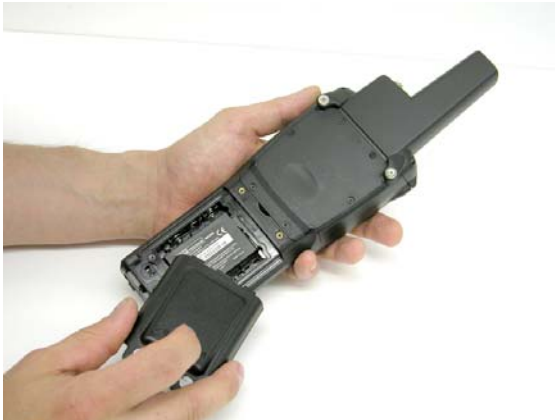
15. Put in the battery and close the battery room
