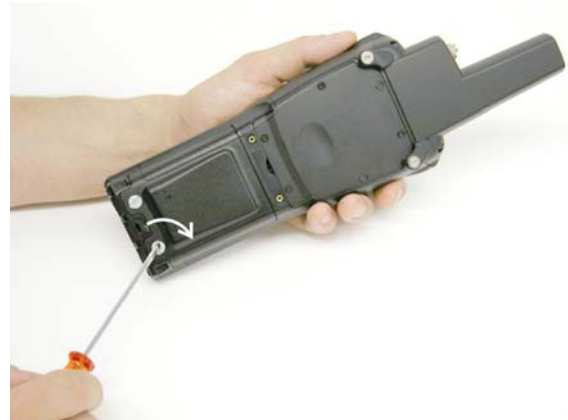
16. by bolting the cover with the screws.
