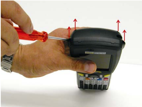
3. Pull out the 4 screws on top
