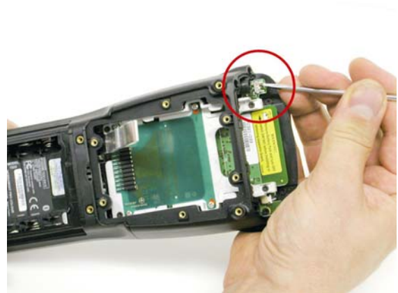
10. Push the SW1401 switch in position ON, again.
