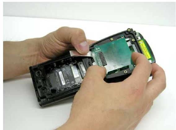
8. Put in the adapter board as shown above.
