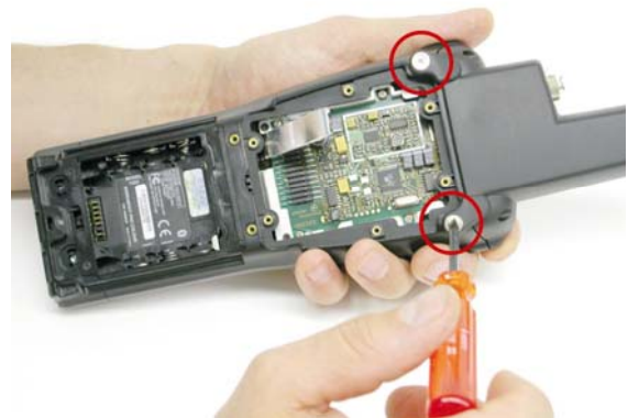
12. and fix it with the 2 added washers and screws.
