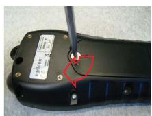
Put the battery cover back in place and turn the screw 90° clockwise. Be aware, that the APR500 housing will only retain its protection class when the battery cover is properly attached.
