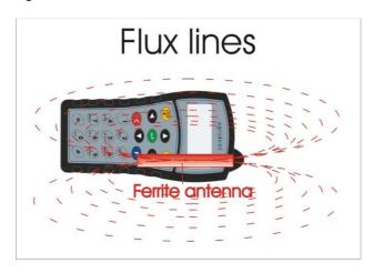
As a result of the flux line characteristics, there is a best reading orientation and a worst reading orientation:
