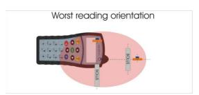
The reading range does not only depend on the transponder orientation but also on the type of transponder. Transponders with a good performance have a better reading distance than low performance tags.
