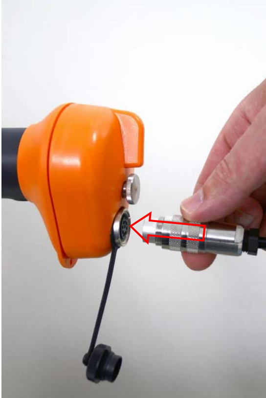
Figure 4: RS232 connection RS232 cable to end cap
