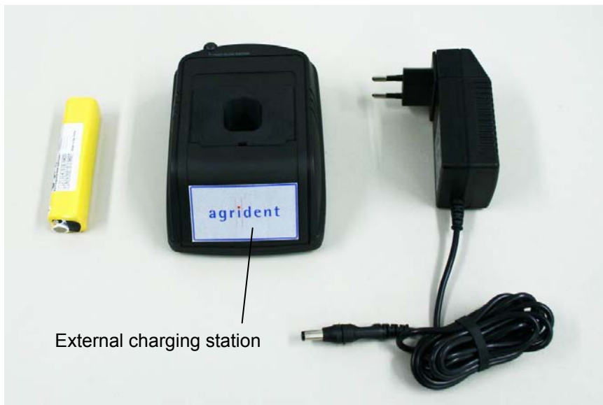
Figure 3: External charging station plus one battery pack
