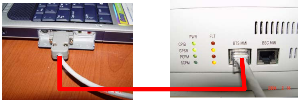
Figure 7-2 - PC to OneRAN Pilot Station Cable Connection Diagram
