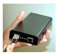
2. Connect the power cable to the 12 VDC power socket on the rear panel, and plug the power adapter into the wall outlet. **Warning**: Use only the power adapter supplied with the AI108 wireless bridge in order to prevent damage.
