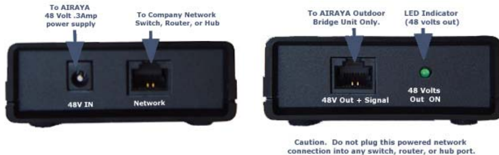
Figure 5. Network and outdoor connection views
