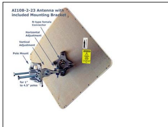
Figure 6. If using 23 dBi directional antennas supplied by AIRAYA, pole mast mounting of the external antennas can be accomplished using the included mounting brackets with full vertical and horizontal adjustment.
