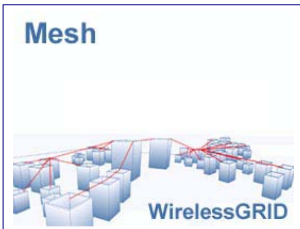
Figure 4. This diagram illustrates the combined use of WirelessGRID backhaul, repeater and multi-point equipment to cover a large geographic area, creating a mesh network.
