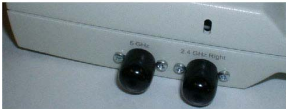
B. 5 GHz/802.11a and 2.4 GHz/802.11b Right External Antennas
