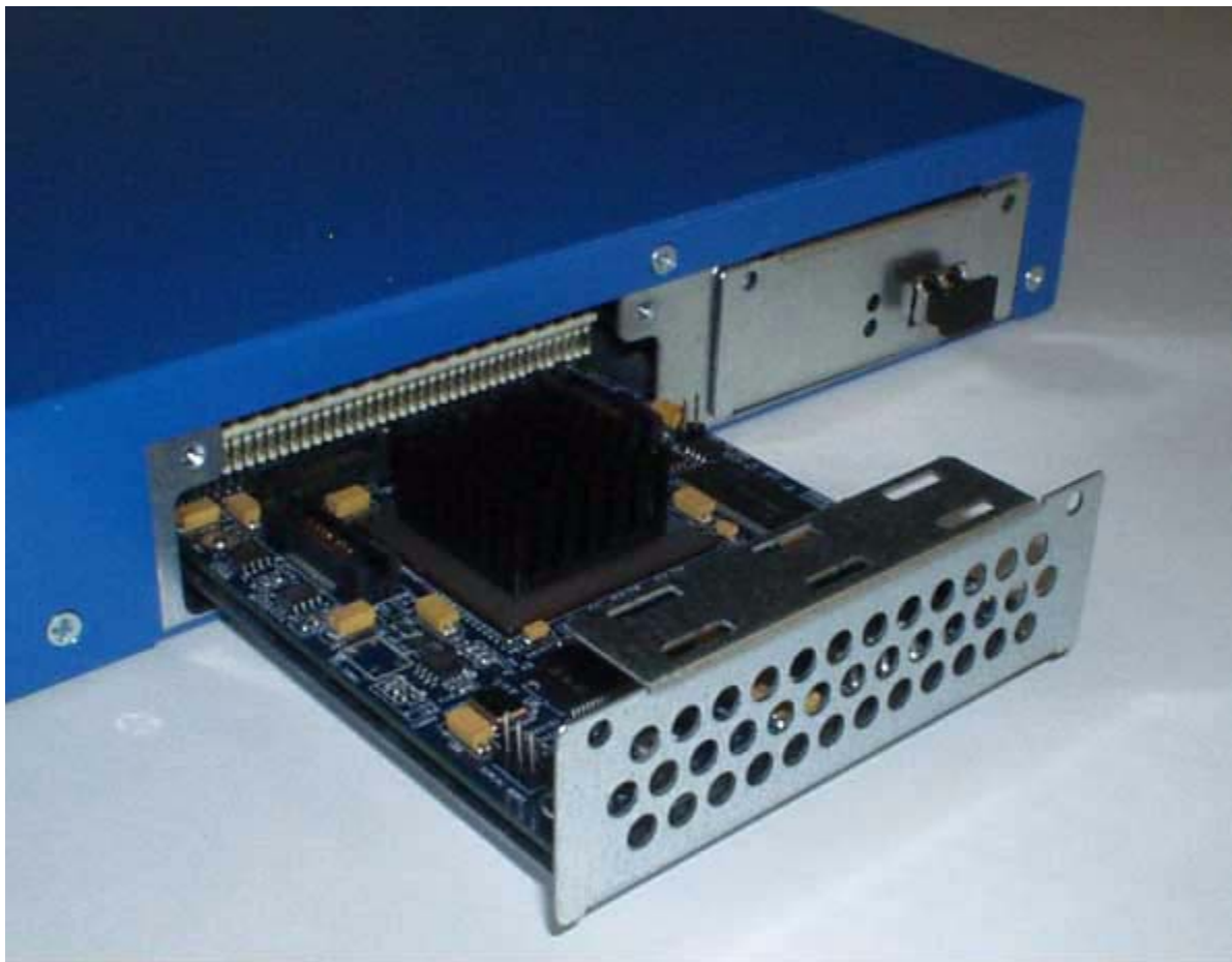
Figure - 4012 and 4024 Airespace Wireless Switch Enhanced Security Module Location
