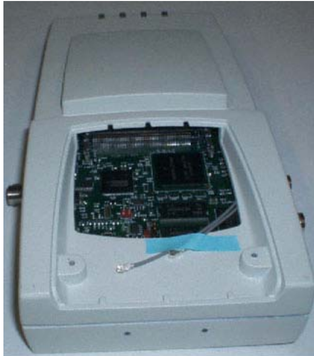
Figure - Airespace AP with Door Removed
