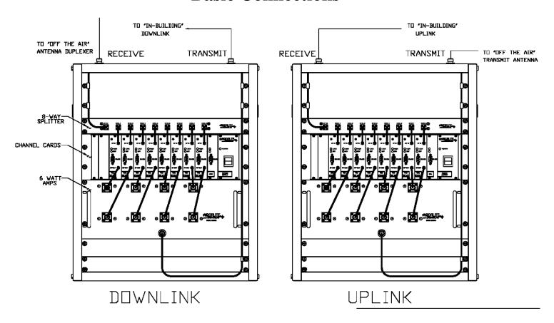
The Basic Connection Diagram shown above, is the proper way the BDA should be connected and once up and running, require minimal to none manual configuration. Connections between cabinets are made through N-Bulkhead connectors located on the top of each cabinet. All programming and adjusting is done through the software and this manual primarily deals with this topic.
