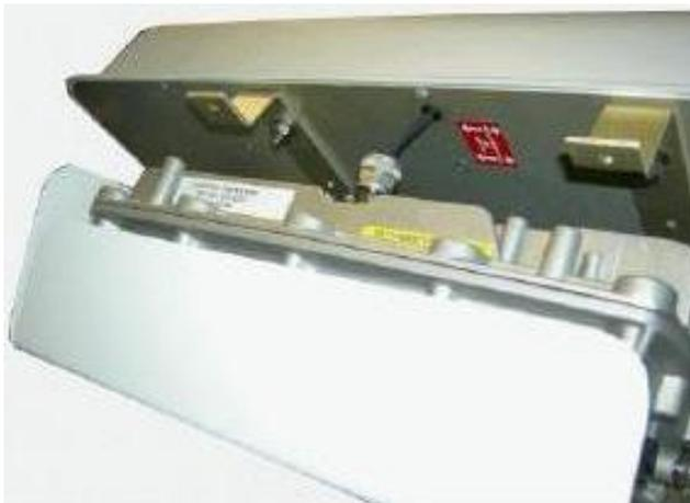
Figure 11 – HiperMAX-micro SCRT antenna RF connection
