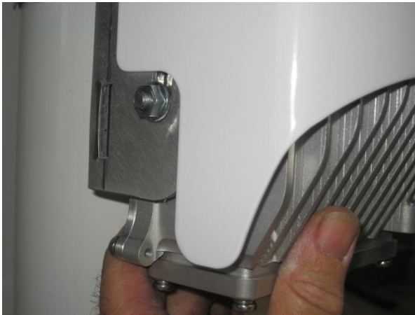
Figure 17 – AirSynergy body engaged in the bottom slots
