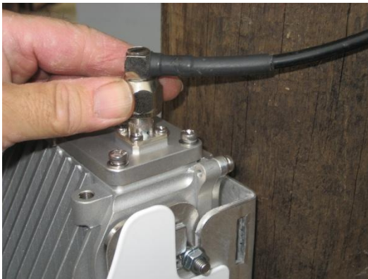
Figure 9 – Connecting the antenna RF cables
