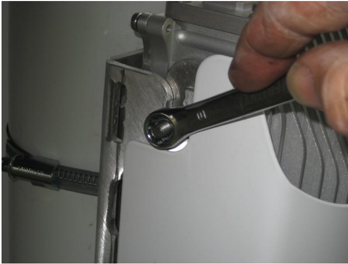
Figure 13 – Tighten flange nuts (4 positions) once the required mounting angle is set
