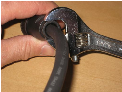
Figure 52 – Assemble the connector and tighten the sealing gland
