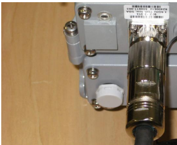
Figure 39 – Attach the power cable to the AirSynergy
