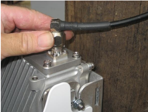
Figure 36 – Connecting the antenna RF cables
