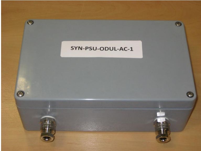
Figure 71 – AirSynergy Mains PSU and enclosure for USA deployments
