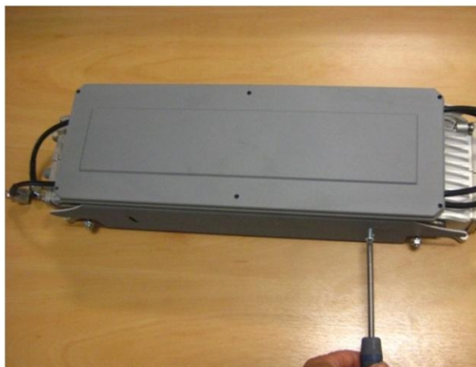
Figure 24 –Fitting the Front mount antenna assembly to AirSynergy
