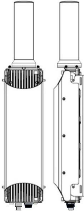
Figure 3– AirSynergy with Switched Beam Antenna
