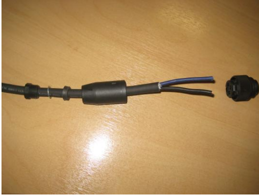
Figure 45 – Cable gland and connector body positioned on the drop cable.
