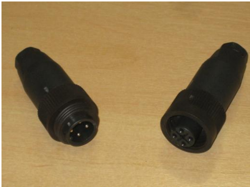
Figure 43 – Water proof power connector with the 2 halves separated
