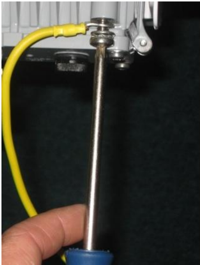
Figure 34– AirSynergy attachment of earthing cable
