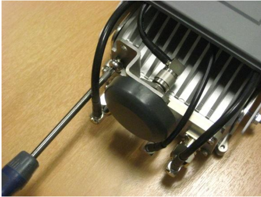
Figure 27 – Assembling the GPS antenna and bracket assembly to AirSynergy
