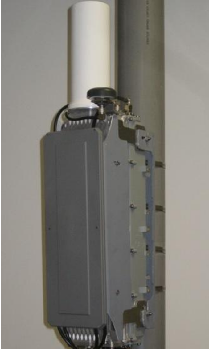
Figure 69 - Back to Back AirSynergy mounted on pole with 4 mounting straps
