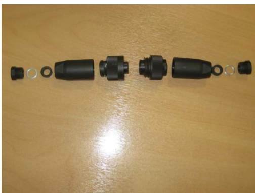
Figure 44 – Waterproof connector dis-assembled ready for installation on the cables
