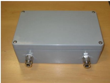
Figure 15 – Enclosed PSU (US requirement)
