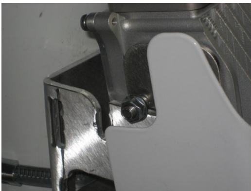
Figure 28 – Lift AirSynergy to top of pole-mount plate
