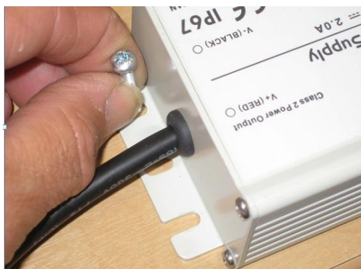
Figure 56 – Fix the PSU into position using self tapping screws
