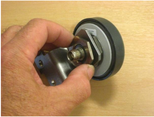
Figure 25 –Fitting the GPS antenna to the mounting bracket
