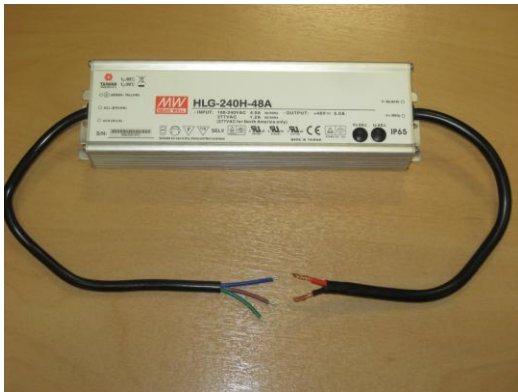
Figure 54 - High power (240W) PSU showing the Mains and low voltage connections
