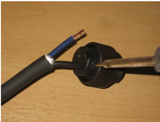
Figure 46 – Fit the cable ends into the connector and secure
