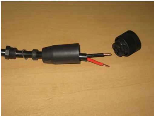
Figure 50 – Prepare the ends of the PSU cable and thread the connector part over the cable
