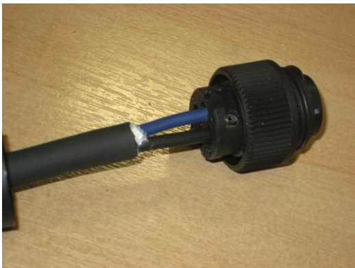
Figure 47 – Male part of connector with both drop cable wires fitted
