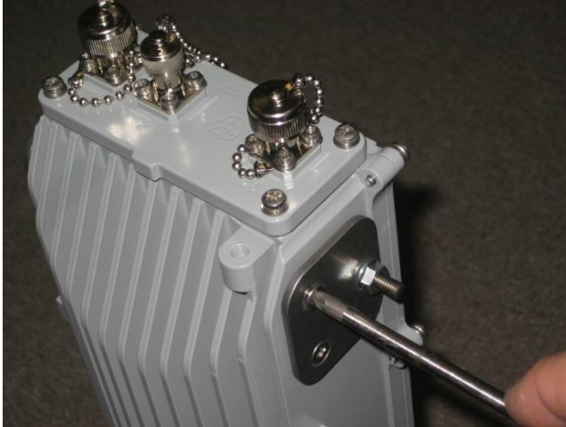
Figure 64 - Removing the existing stud mounting plates
