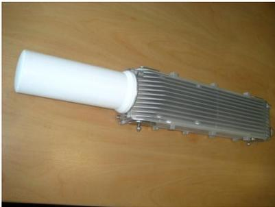
Figure 8 – AirSynergy unit with Switched Beam Antenna (factory fitted)
