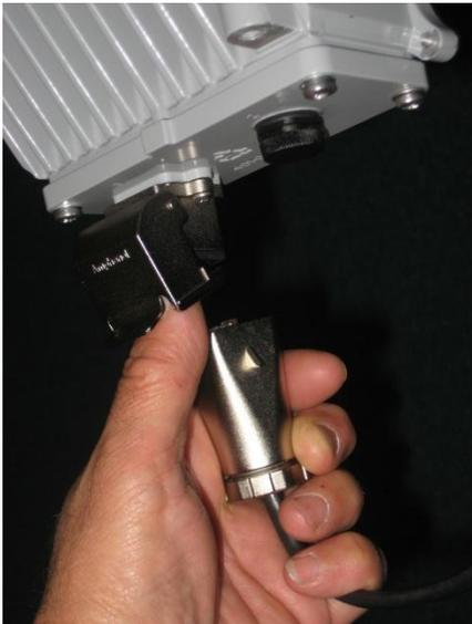
**Figure 36 – Attach PoE drop cable to the AirSynergy**
