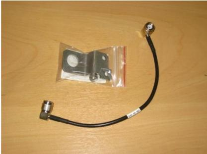
**Figure 14 – GPS antenna mounting kit**
