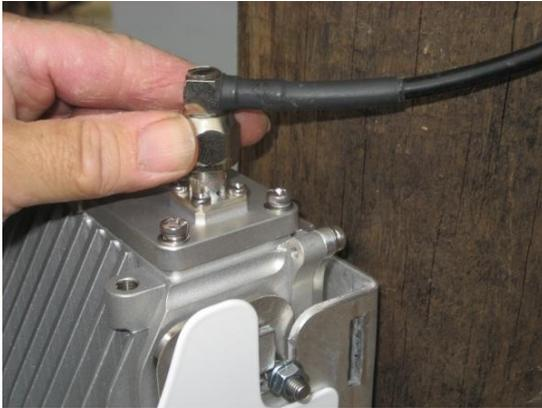
Figure 33 – Connecting the antenna RF cables
