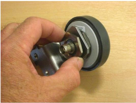
Figure 22 –Fitting the GPS antenna to the mounting bracket
