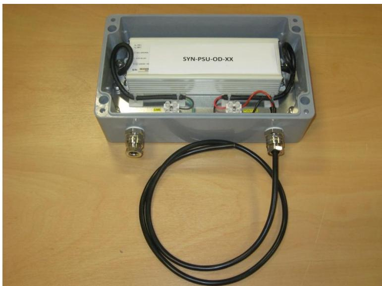
**Figure 70 – 48V DC cable attached ready for connection to the PoE injector**
