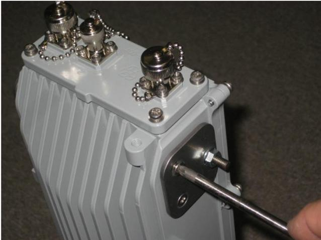
**Figure 62 - Removing the existing stud mounting plates**
