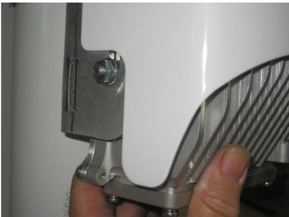
Figure 28 – AirSynergy body engaged in the bottom slots
