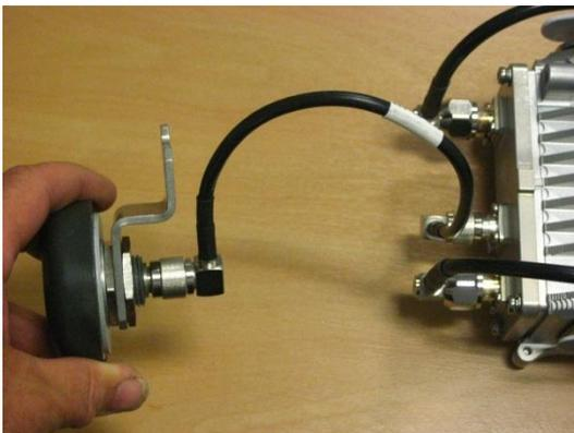
Figure 23 –GPS antenna cable connected
