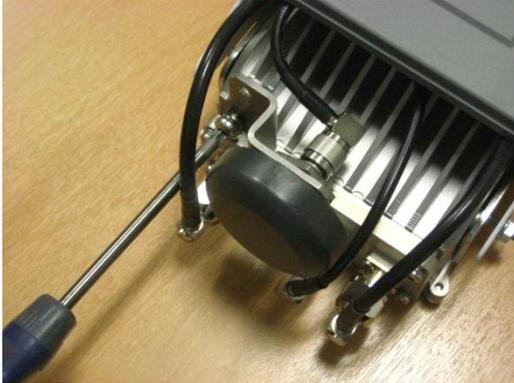
Figure 24 – Assembling the GPS antenna and bracket assembly to AirSynergy
