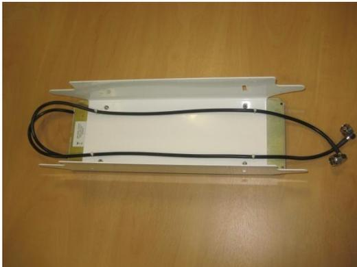
**Figure 20 – Fixing the front mount antenna to the mounting plate**
