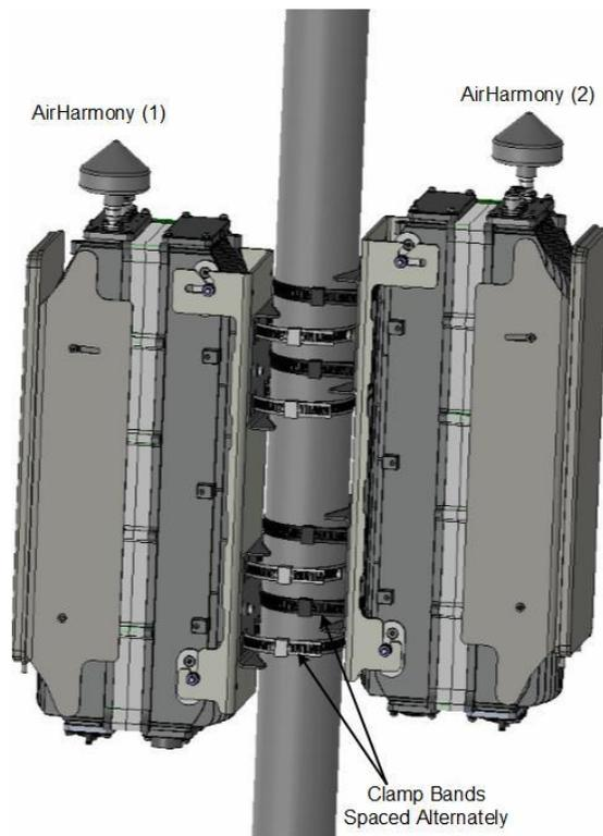
The difference in height between the installed units after installation will be 40mm.
