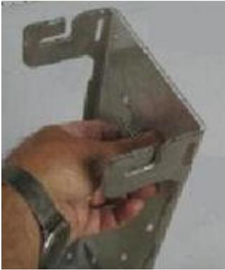
2. Mark the wall through the holes on the wall mount at the required height.
