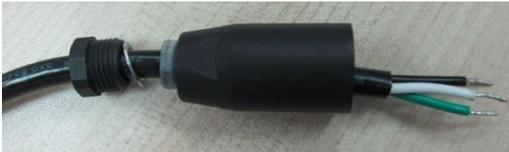
4. Insert and secure the **white** wire into position **1** and the **black** wire into position **2** and **green** wire into position  $\perp$  (earth ground).
