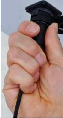
**Note:** The shell should be hand tightened only. Do NOT use tools to tighten the shell.
