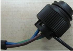
6. Insert and secure the **brown** wire into position **1** and the **blue** wire into position **2** and **green** wire into position  $\perp$  (earth ground).
