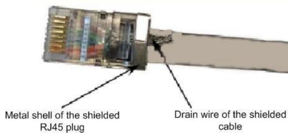
15. Seat the RJ45 connector plug securely into the body cavity.
