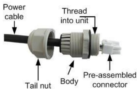
**Caution:** Do not over tighten the gland connector or the tail nut. The gland nut should be tightened to a torque of no more than 3.3 Nm (2.43 lb-ft) max.
