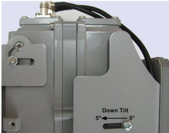
3. After adjusting to the required tilt amount tighten both flange nuts and both screws. The antenna has an electrical fixed down-tilt of 1°.
