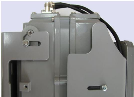
3. With the studs engaged in the top slots raise the unit slightly until the bottom studs also drop into their respective slots.
