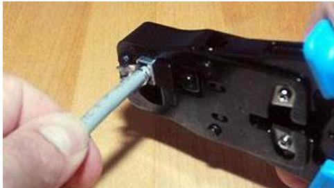
**Note:** All pins should be fully compressed and of equal height after crimping.
