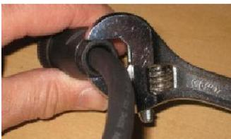
6. Fasten the 2 parts of the connector together and tighten to make a waterproof seal.
