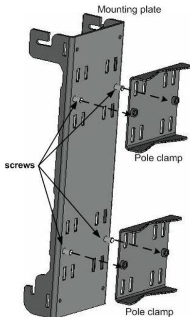
2. Insert the clamp straps through the slots in the mounting plate passing them through the pole clamps.
