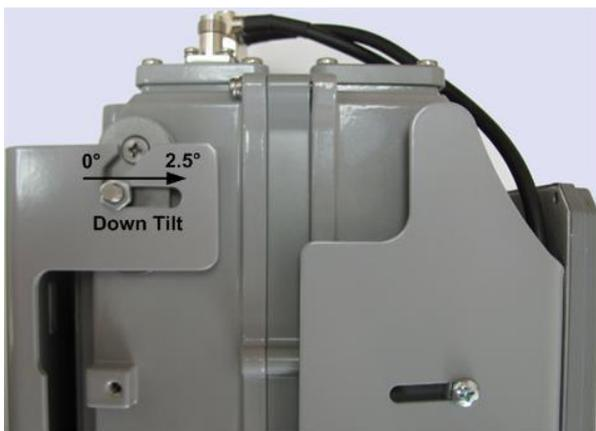
2. Slightly loosen the upper screws (2) where the front mount antenna is fixed to the unit.
