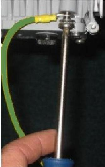
2. Connect the ground cable to the protection ground bar using suitable crimp lugs. Alternatively use a clamp to bond the ground cable to the mounting pole or to the tower structure.
