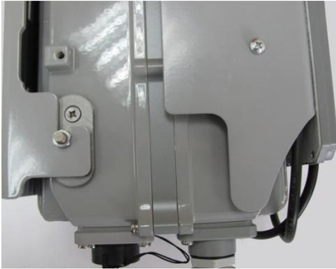
4. Tighten the flange nuts (4 places) to the required degree of down-tilt.
