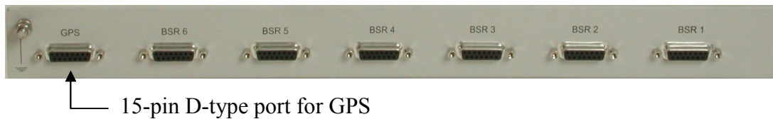
Figure 10-2: BSDU rear panel showing GPS port
