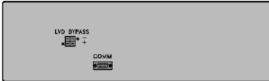
Figure 7-12: DC Distribution Rack rear view
