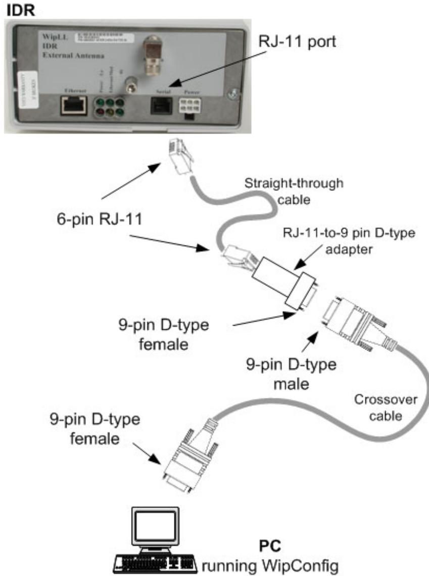
Figure 12-13: IDR-to-PC serial cable connections
