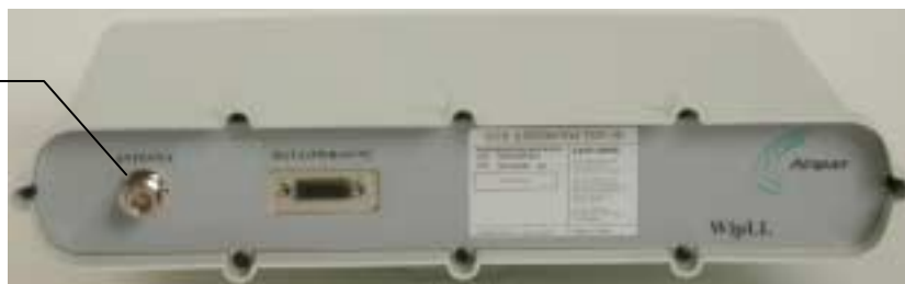
Figure 4-9: BSR model with N-type antenna connector
