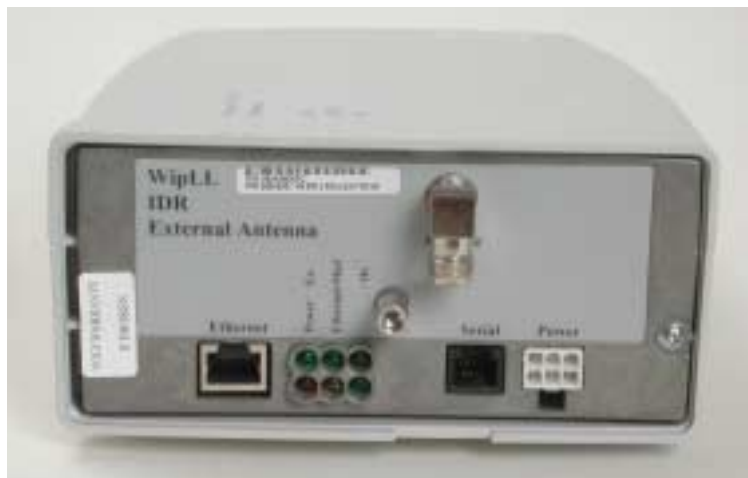
Figure 10-2: IDR with lower cover removed exposing ports
