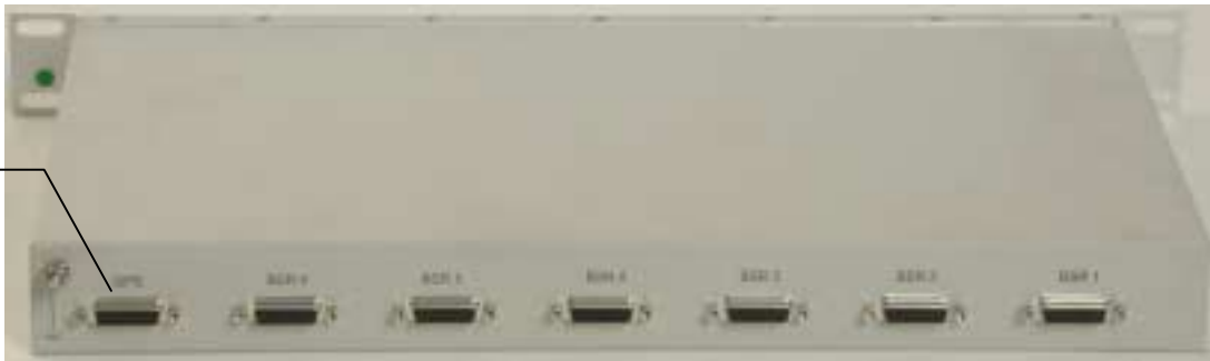
Figure 6-2: BSDU rear panel showing GPS port
