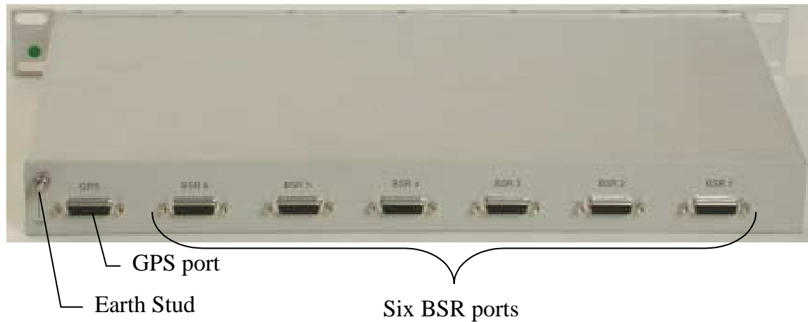
Figure 5-5: BSDU rear panel
