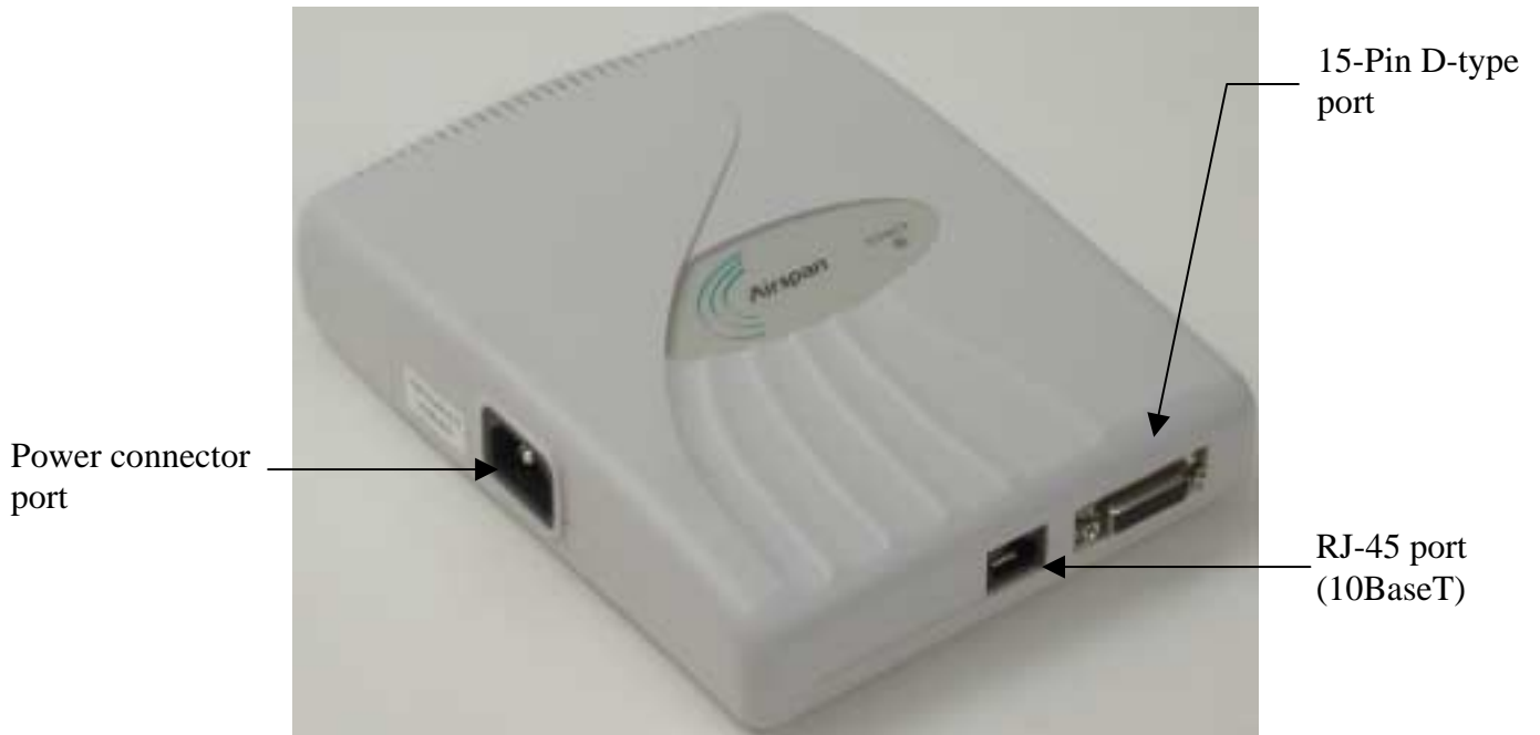
Figure 9-3: SDA-1 (front, side, and top panels)
