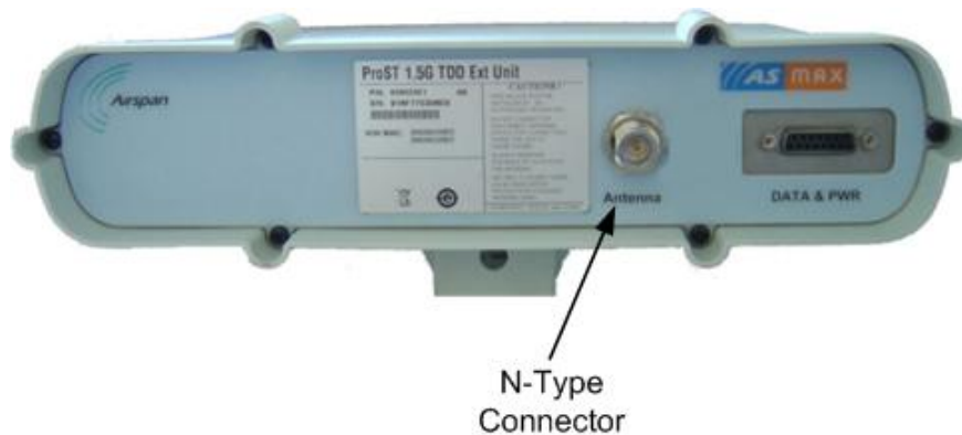
Figure 5 - ProST with external antenna
