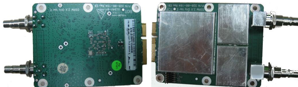
Figure 2 – SSRM PCIe module
