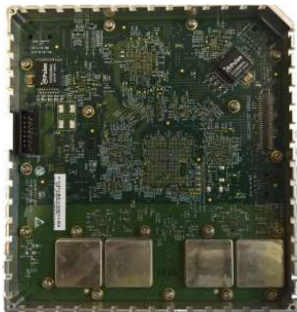
Figure 3: AU540 eNB B41 module inside housousing (w/o cover)
