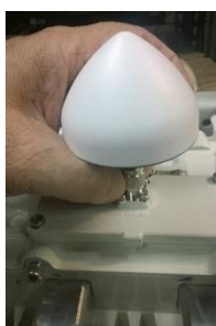
Figure 18: Attaching GPS antenna to unit
