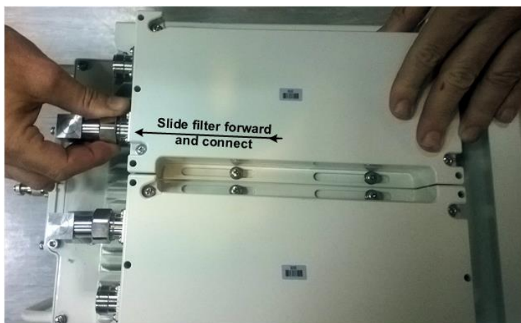
Figure 15: Align and fit second filter to connector
