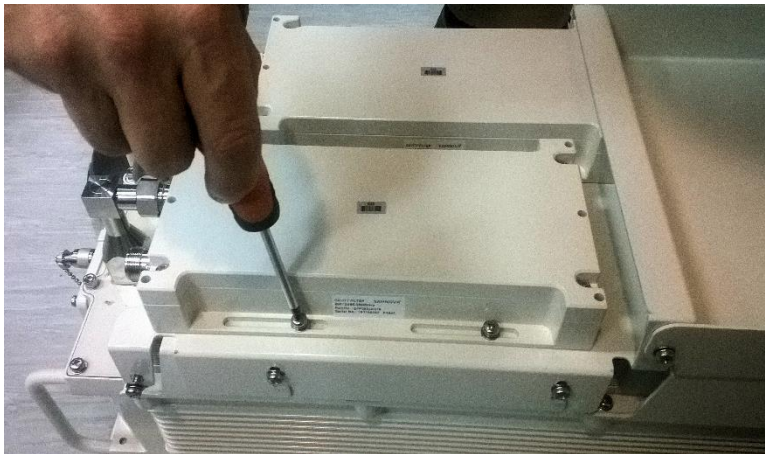
Figure 14: Tighten screws on filter
