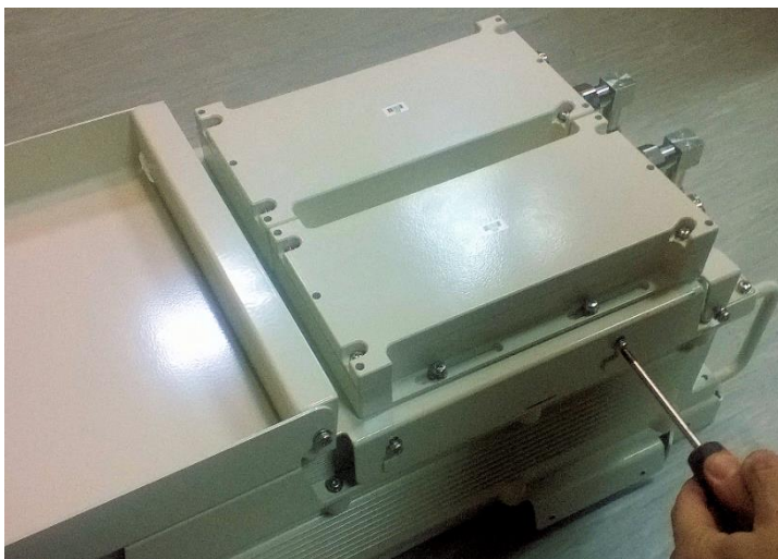
Figure 16: Tighten filter bridge screws on Sun-Shield
