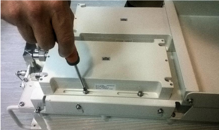
Figure 20: Tighten screws on filter
