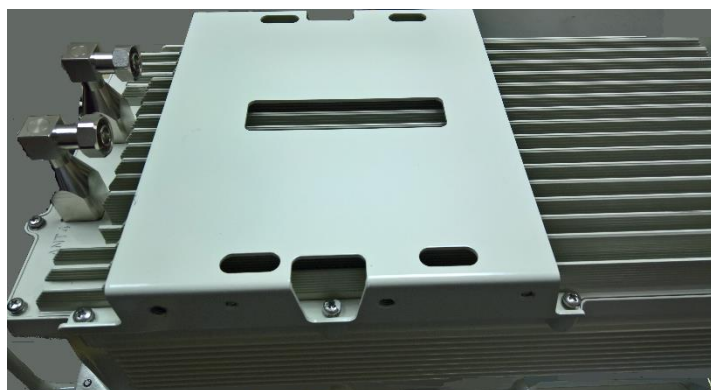
Figure 6: AirHarmony-4400 - in Horizontal Position prior to Rear External Filters Set Assembly
