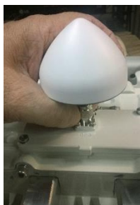
Figure 24: Attaching GPS antenna to unit
