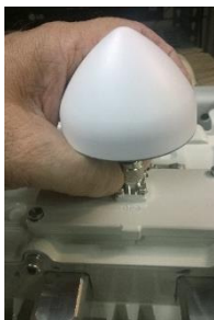
Figure 6: Attaching GPS antenna to unit
