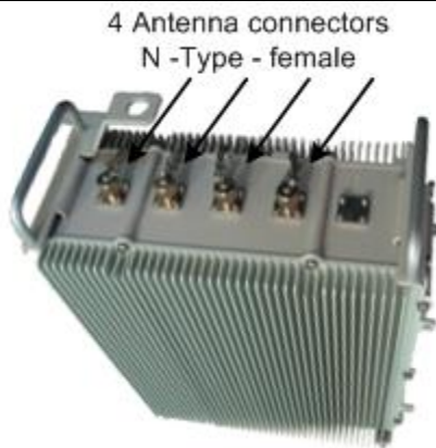
Figure 28 – Air4G External Antenna Configuration
