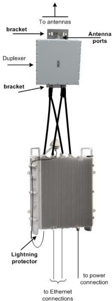
Figure 40 - Pole Mounted external Duplexer.
