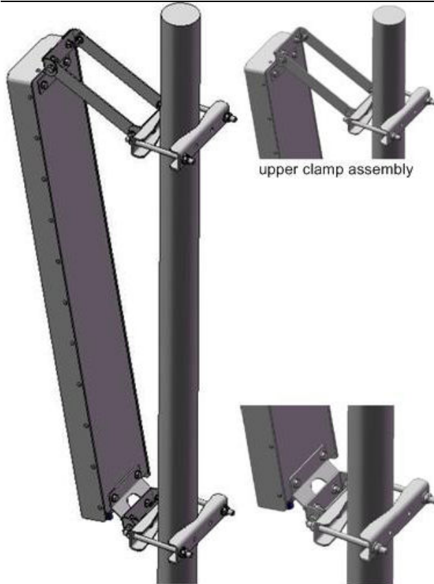
Figure 32 - Adjustable Mounting Kit, with 'V' Blocks
