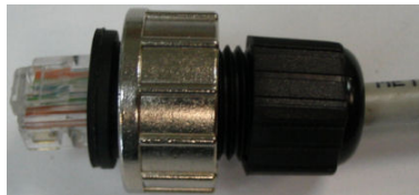
Figure 54 – Ethernet environmental connector assembly
