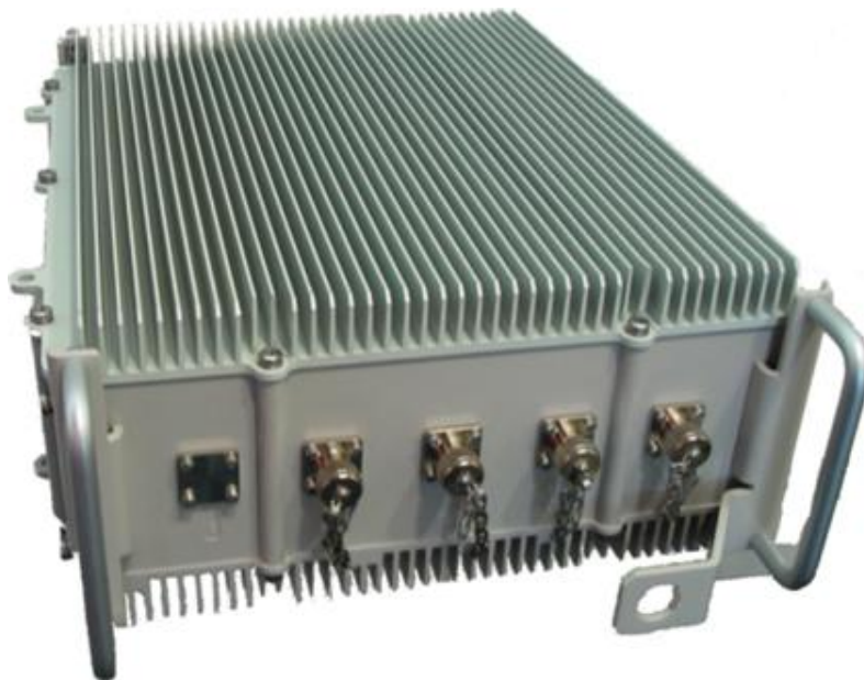
Figure 7 – Air4G Base Station Unit, RF ports
