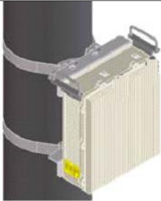
Figure 17 – Pole Mounted Air4G
