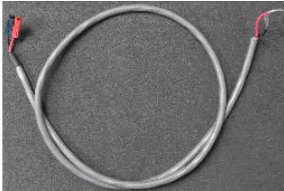
Figure 58 - BSDU to DC cable
