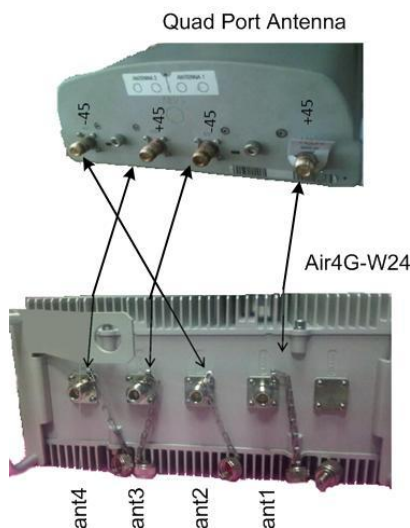
Figure 34 - Quad port antenna connection – 1
