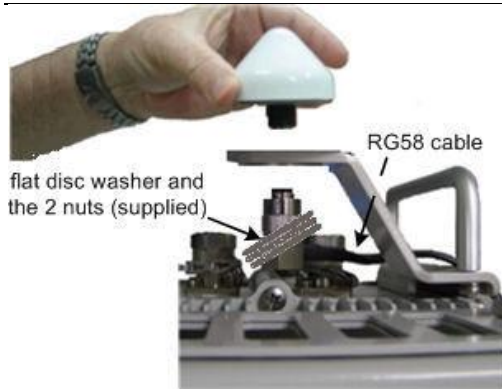
Figure 37 - Attach GPS antenna to RG58 cable
