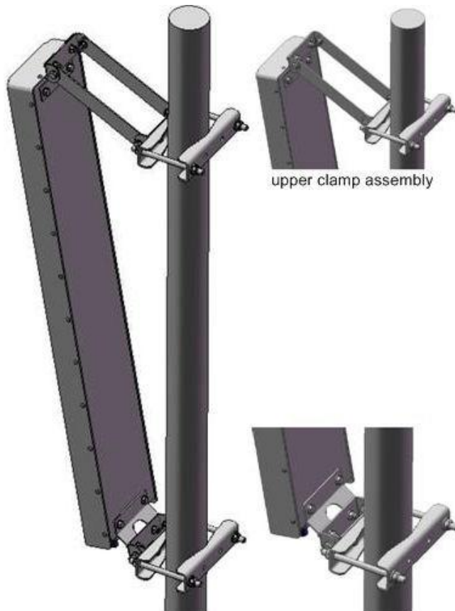
Figure 27 - Adjustable Mounting Kit, with Snaplock Stainless Steel Bands
