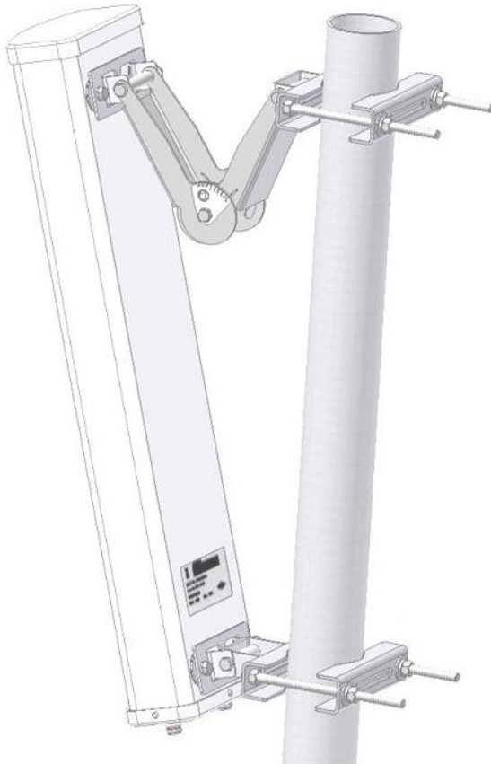
Figure 25 - Air4G-W24 Antenna Dual Slant Mast Mount Configuration
