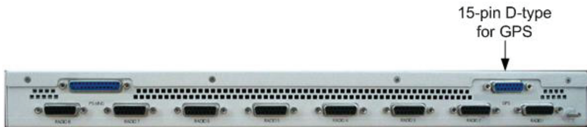
BSDU rear panel showing GPS port
