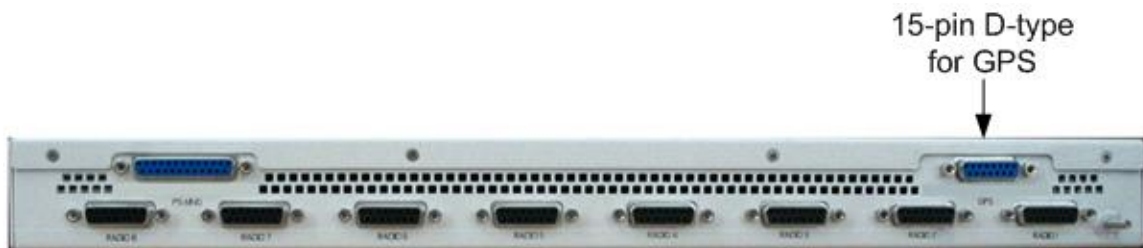
BSDU rear panel showing GPS port
