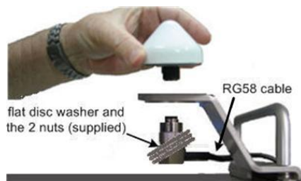
Figure 15 - Attach GPS antenna to RG58 cable
