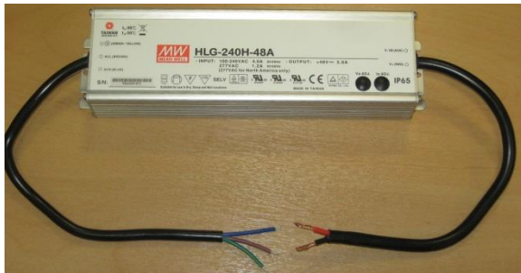
Figure 46 - High power (240W) PSU – used for dual AirSynergy installations
