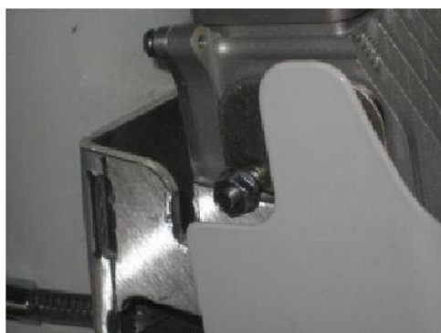
Figure 23 - Lift unit to top of mounting plate
