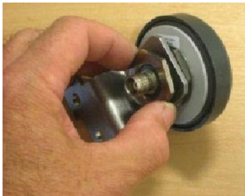
Figure 20 - attaching GPS antenna to mounting bracket
