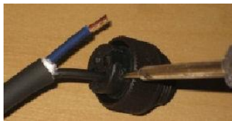
Figure 38 - secure cable to connector
