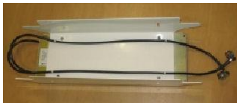
Figure 18 - attaching front mounted antenna to mounting plate
