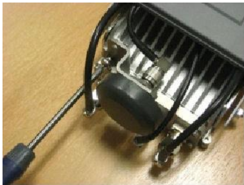
Figure 22 - Assembling GPS antenna with bracket to AirSynergy
