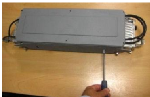
Figure 19 – Attaching front mount antenna assembly to AirSynergy
