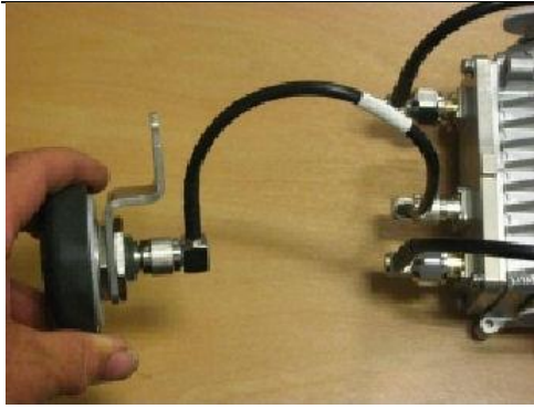
Figure 21 - GPS antenna cable connected
