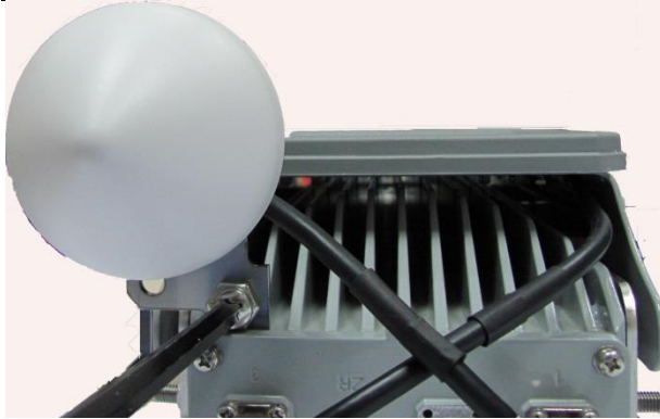
Figure 20 - Attaching the GPS antenna assembly to AirSynergy
