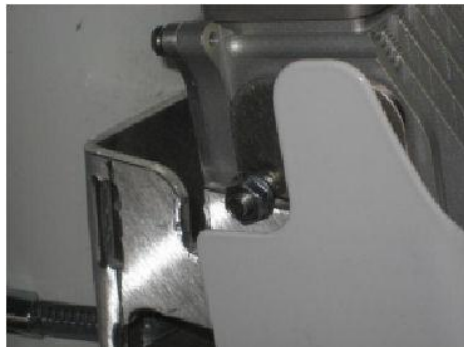
Figure 21 - Lift unit to top of mounting plate
