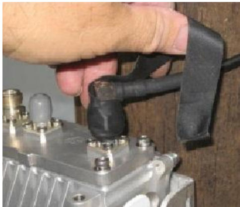
Figure 30 - weather-proof the connection - external antenna
