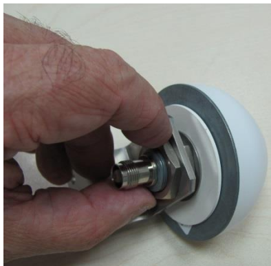
Figure 19 - attaching GPS antenna to mounting bracket
