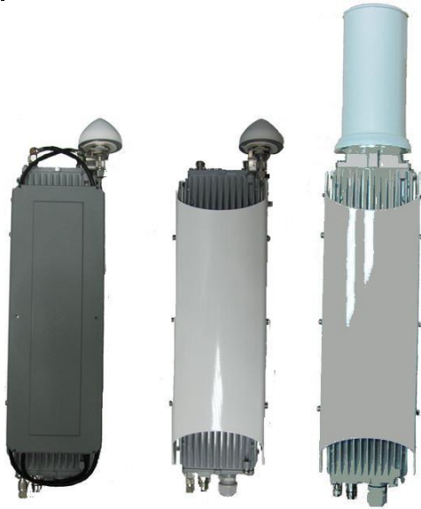
Figure 4 - AirSynergy 2000 assembled with: Front Mount antenna, sunshield, SBA and sunshield
