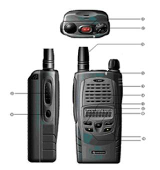
Emergency Key Power on / off and Volume Control Switch Turn the transceiver on by rotating power on / off and volume control switch clockwise and control the volume. Helical Antenna.
