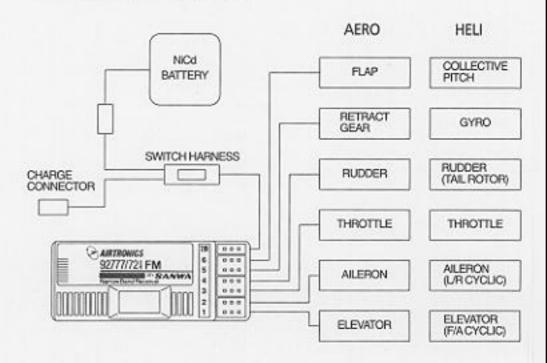
The above diagram show how to connect the components of your RD6000 system together. At this point, your objective is to get the system operating on your workbench. Once connected, you must then refer to the corresponding diagram for your system, i.e., either AERO or HELI showing the transmitter control sticks' function.
