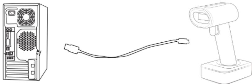
B: Base charges and transfers data synchronously: When base connected to USB cable, the other end is plugged into computer ,
