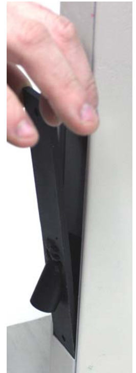
FIG. 5A: MORTISE DRILL JIG PLACEMENT
