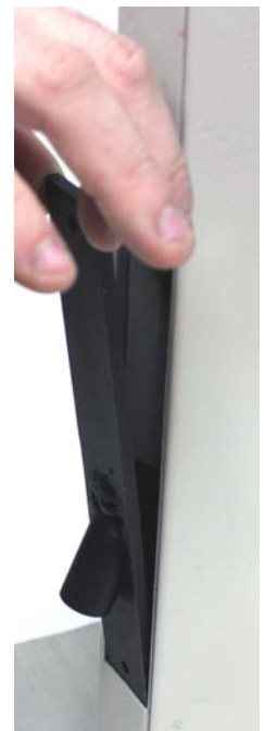
FIG. 11A: MORTISE DRILL JIG PLACEMENT
