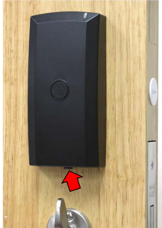
FIG. 19A: INSERT "DOG POINT" SCREW HERE
