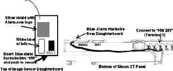
5. Route Daughterboard Antenna- It is important to be sure that daughterboard antenna is pulled away from the Alarm.com module. Follow the panel-specific antenna routing guidelines to optimize sensor range.
