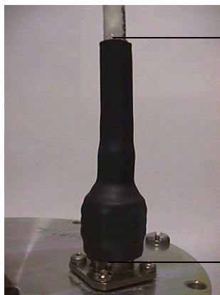
Figure 27 – Connecting the "N" connector with the thermoshrinkable sleeve
